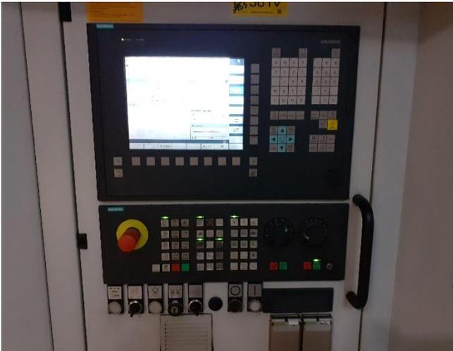
*Control Sinumerik 840D Powerline PCU50 HMI Advanced*
