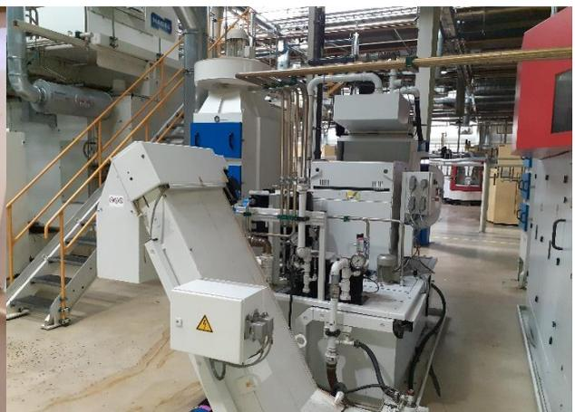
*Coolant device and chips conveyor*
